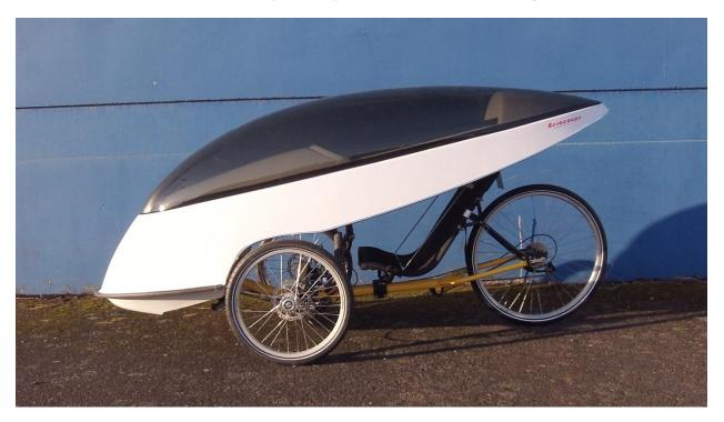
The **Blue Sky Design Aerocoupe Speeder Fairing** is designed to be an affordable accessory for "Cyclecar" (Tadpole) three wheeled recumbent human powered vehicles (HPV). It can substantially improve aerodynamic efficiency, weather protection and visibility in traffic. This Fairing can be removed with one bolt.
